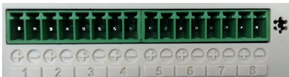
Figure 3-3 Thermocouple Terminals
