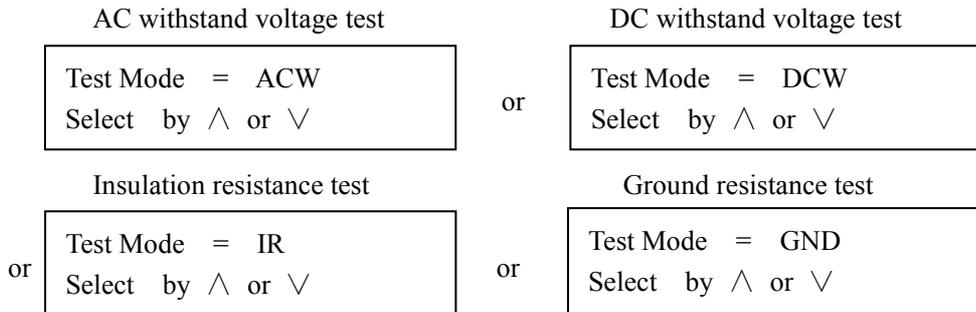
Please use the "+" or "-" key on the panel to enter the test mode to be set: ACW, DCW, IR or GND.
