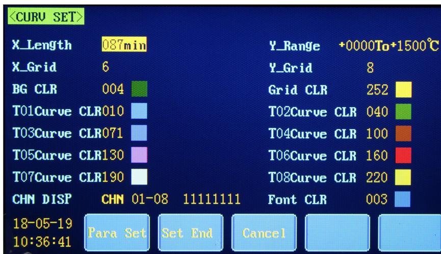
X axis length: X axis time value, 1min~999min can be set freely.
